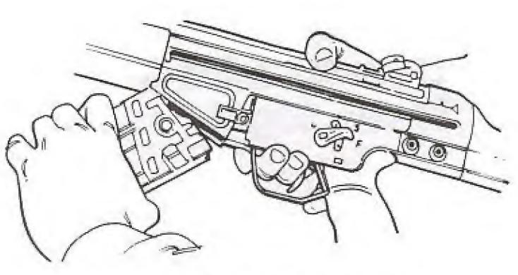
4. Insert the magazine into the magazine well. The magazine should be inserted, front end first with a slight bottom-forward cant, then rolling the rear of the magazine back into place. When the distinctive "click" of the magazine catch is heard, the magazine is engaged.
